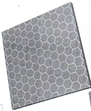
Largest and smallest hexagon grid top contact for the 1mm 2 Silicon solar cell investigated in this study.
