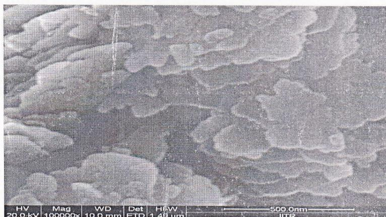
Fig. 7 SEM image of the  $\text{Ca}_2\text{Al}_2\text{SiO}_7:\text{Ce}^{3+}$  (2mol %) phosphor
