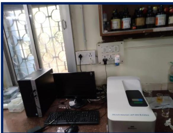
Zeta potential is a measurement based on the charges on the particles in a suspension or emulsion. A zeta potential analyzer does the measurements
