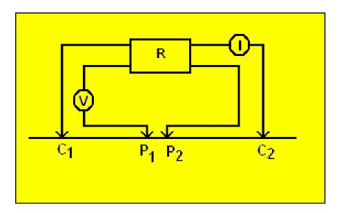
The formula for measuring the electrical resistivity (apparent) is
