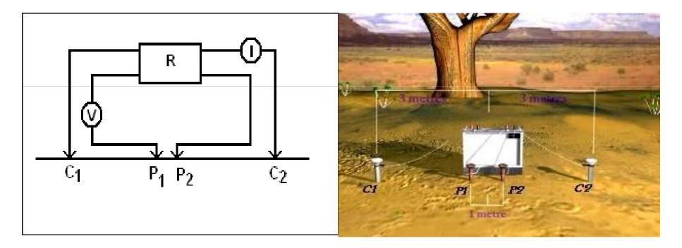
➤The Resistivity value so obtained is termed as Apparent Resistivity which is the characteristic of the subsurface formation under investigation.
