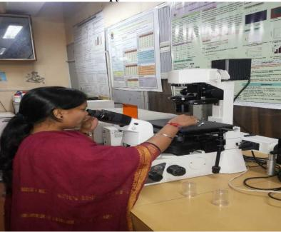
A fluorescence microscope is an optical microscope that uses fluorescence and phosphorescence instead of, or in addition to, reflection and absorption to study properties of organic or inorganic substances. A fluorescence microscope is much the same as a
