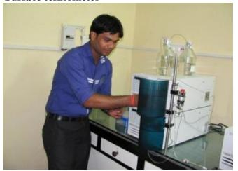
A tensiometer as it applies to physics is a measuring instrument used to measure the surface tension of liquids or surfaces. Tensiometers are used in research and development laboratories to determine the surface tension of liquids like coatings, lacquers or adhesives. A further application field of tensiometers is the monitoring of industrial production processes like parts cleaning or electroplating. Surface tension measurements are done using either force or optical
