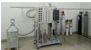
Fabrication of Experimental Setup High pressure fixed bed micro reactor with additional setup
