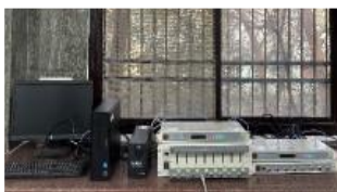
Battery Analyzer 16-Channel, 5 Amps, 5 Volts
