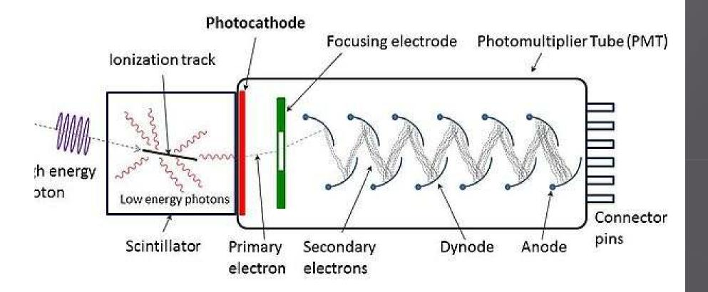
PMT detector is attached to an amplifier and other electronic equipment to count signals.
